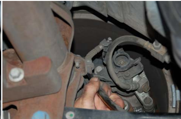
Disconnect cable from caliper
