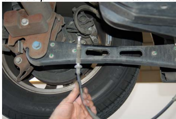
Pull cable through control arm
