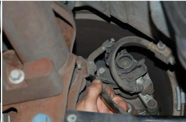
**Disconnect cable from caliper**
