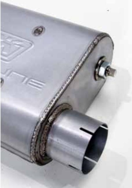
allowing users to adjust sound levels. Adjust inward for a quieter sound, and outward for a louder one.
