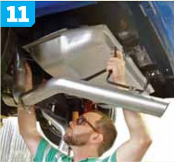
Christ also helped install the over-axle pipes and tailpipes. Using the L-brackets, we secured the tailpipes to the rubber exhaust hangers behind the rear bumper.
