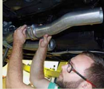
Here, Christ fits and installs the new mufflers. BBK includes an assortment of clamps and hangers to properly mount the mufflers.
