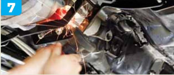
« Due to the extensive customization of our build, certain parts needed to be modified in order to fit. We needed to shave part of the crossmember in order to properly fit the X-style mid-pipe.
